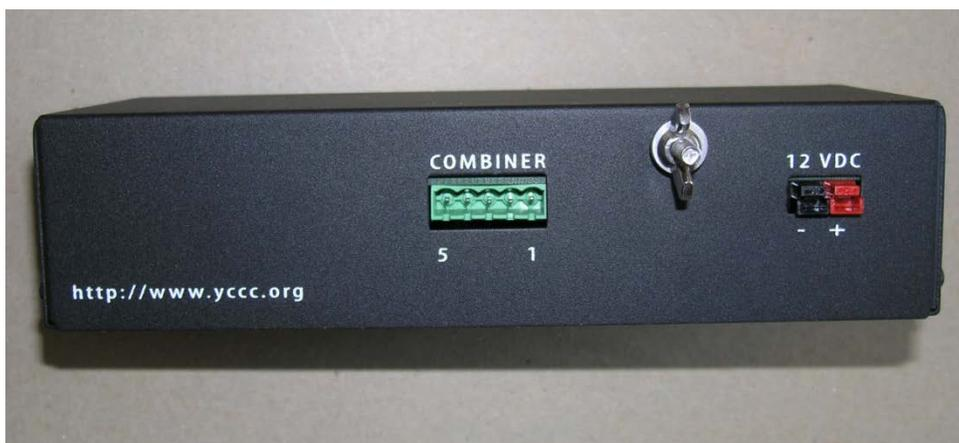
*Figure 34. Rear side of finished direction controller unit*
