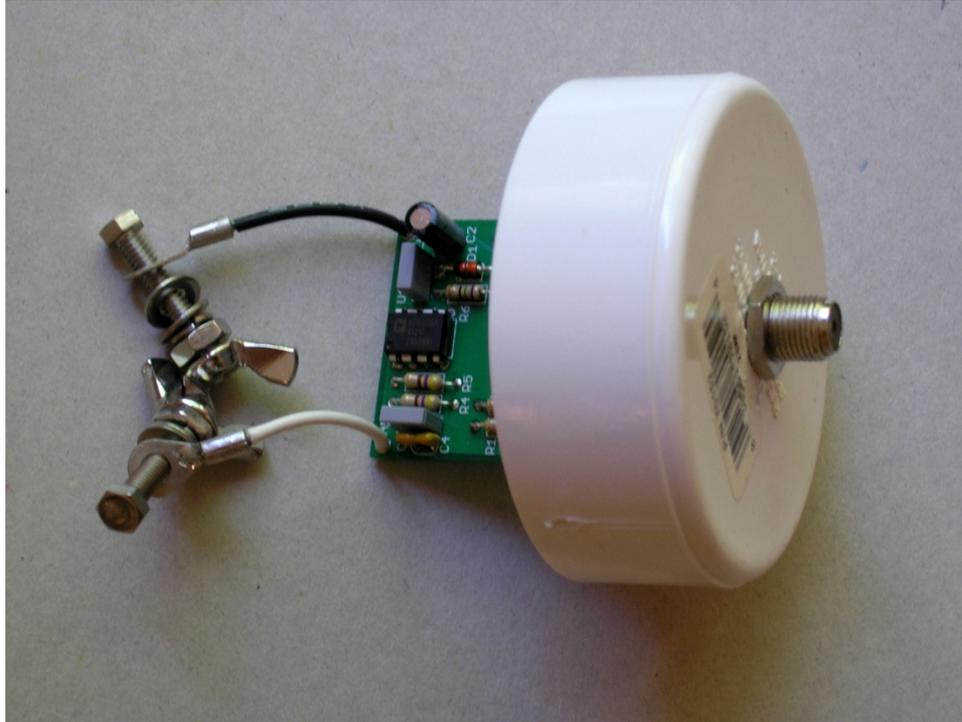
*Figure 12. Preparation of end cap for preamplifier enclosure*
